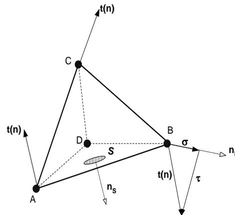
Figure 8. In VTK, a normal vector is defined directly at a surface e.g.,  $\mathbf{n}_S$  at surface S, and tensor attributes is a property of point or grid, e.g., point or grid B
