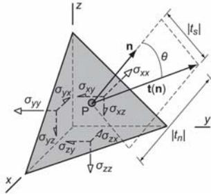
Figure 2. Diagram of traction vector  $\mathbf{t}(\mathbf{n})$  and stress state  $\sigma_{ij}$  at point P which is located on the specific surface. Here, subscripts  $i$  and  $j$  are defined by  $x$ ,  $y$ , and  $z$
