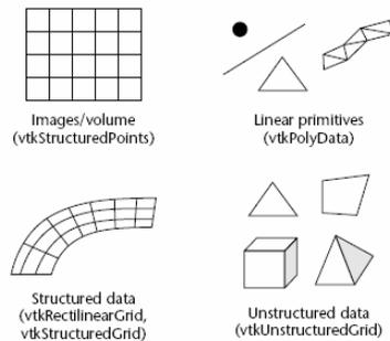
Figure 6. Type of data set supported by VTK (see VTK User's Guide)
