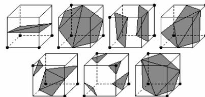
Figure 1. The cutting processes using marching cube show several possibilities to obtain cut surfaces from 3-D objects numerically
