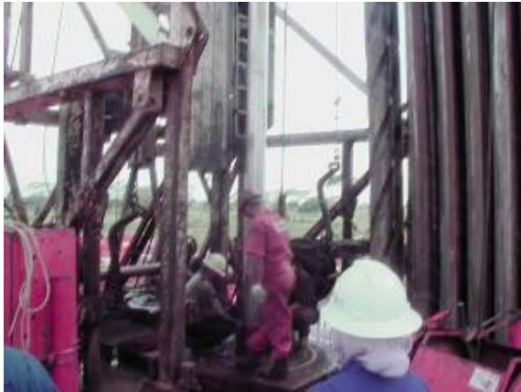
Picture 5. Making up LWD tools on the rig floor
