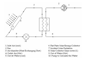
Figure 1. Schematic diagram of solar heating of air
