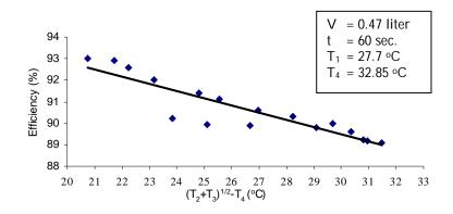
Figure 2. Collector efficiency relation with mean water temperature
