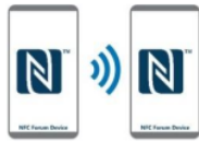
Gambar 2. Mode operasi peer to peer
