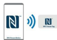
Gambar 1. Mode operasi reader/writer
