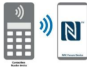
Gambar 3. Mode operasi card emulation
