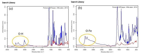
1500cm-1 at Figure 3b wider than Figure 3a, because the change in bonding from C-N  $Na_2H_2EDTA.2H_2O$  to C-Fe bond on Fe-EDTA.
