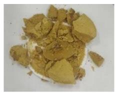
Figure 2. Fe-EDTA synthetic result
