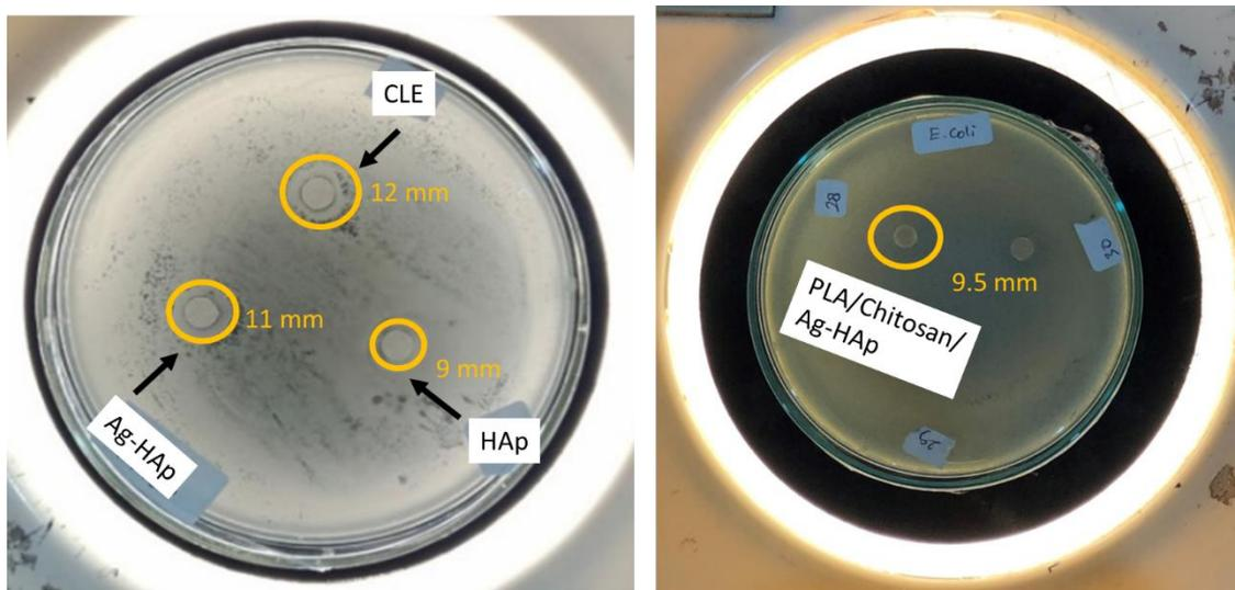
Figure 8. Images from the antibacterial test against *E. coli*
