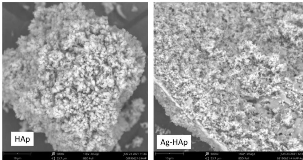
Figure 5. SEM image of HAp and Ag-HAp
