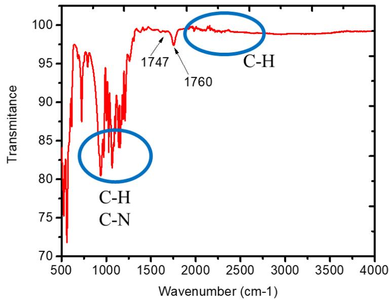
Figure 7. FTIR spectrum of PLA/Chitosan/Ag-HAp
