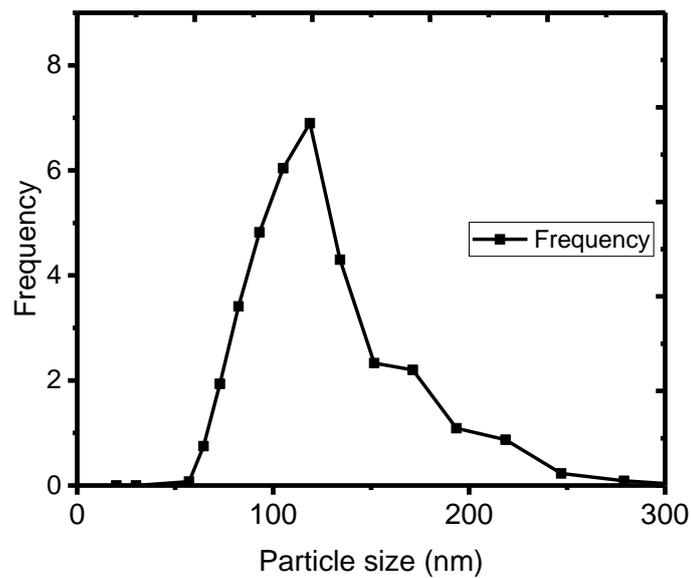
**Figure 3.** Particle size distribution of Ag NPs
