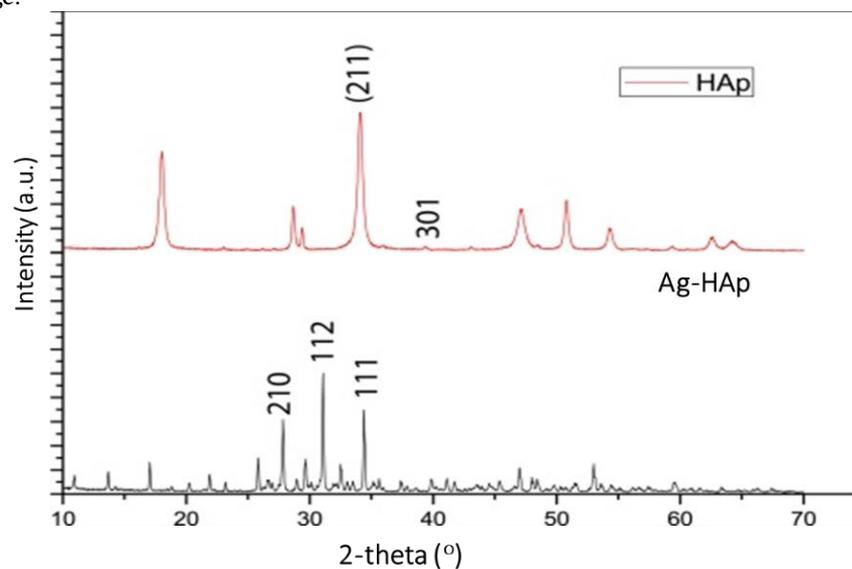
**Figure 4.** XRD pattern of HAp and Ag-HAp
