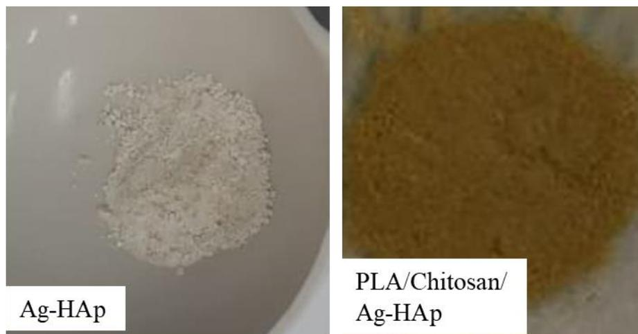
Figure 6. Physical appearance of Ag-HAp and PLA/Chitosan/Ag-HAp
