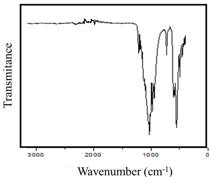
**Figure 2.** FTIR spectra of AgNPs
