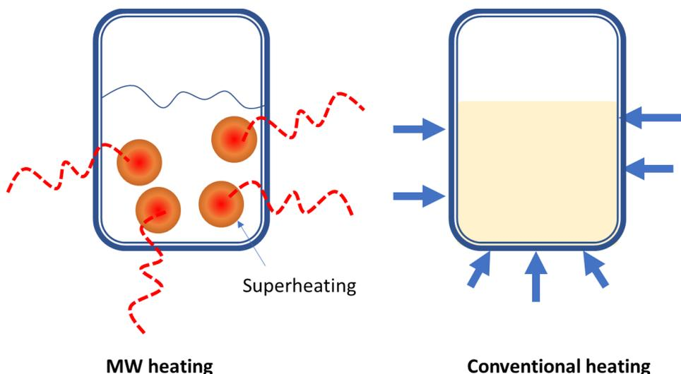
**Figure 2.** Differences in heat flow patterns in regular heating and MW
