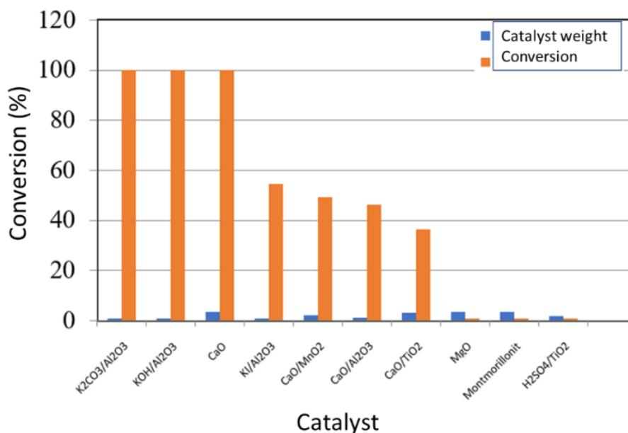
**Figure 5.** Effect of catalyst types on the methyl ester yield of sunflower seed oil (Reaction conditions of methanol: oil ratio = 16:1; Catalyst 10 wt.%; reaction time 2 hours, temperature 70 °C)
