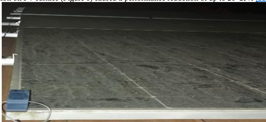
Figure 6. PV Module Surface Covered by Dust at the Site
