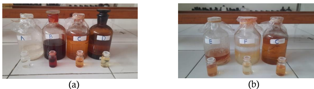
Figure 5. Visual characteristics of synthesized phenol–formaldehyde syntans at varying molar ratios, showing the effect of phenol and formaldehyde composition on color and homogeneity.
