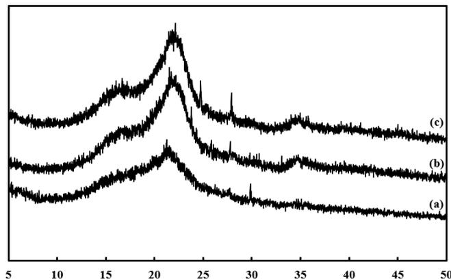
Figure 2. XRD analysis results (a) Pineapple leaves before delignification (b) Pineapple leaves after 5% NaOH delignification, and (c) Pineapple leaves after 9% NaOH delignification.
