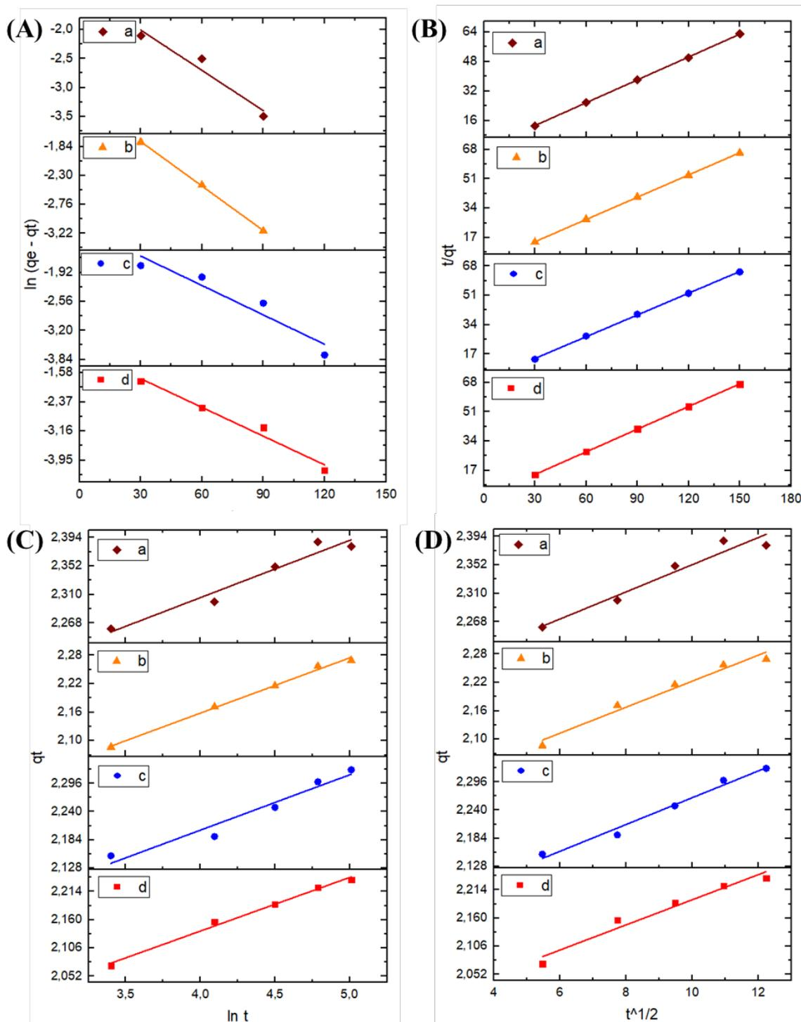
Figure 5. Fitting curves of different kinetic equations of MB adsorption by adsorbent (A) 9% NaOH delignification, cell-PVA; (B) 5% NaOH delignification, cell-PVA; (C) 9% NaOH delignification, cell; (D) 5% NaOH delignification, cell) (inset: a. Pseudo-first-order kinetics
