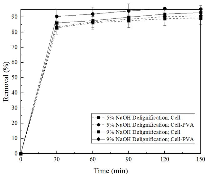
Figure 4. Effect of contact time on methylene blue dye removal.
