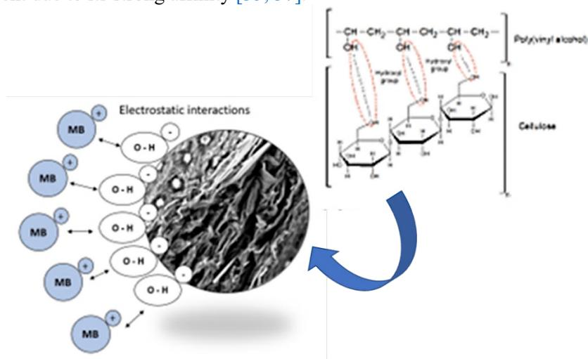
Figure 6. Schematic of adsorption mechanism.
