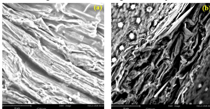
Figure 3. SEM analysis results with 2500x magnification (a) Cellulose (5% NaOH delignification) - PVA and (b) Cellulose (9% NaOH delignification) - PVA
