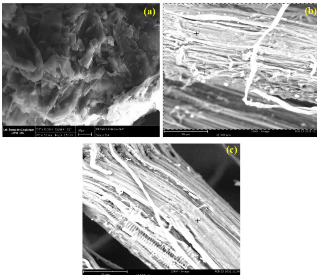
Figure 1. Results of SEM analysis with 2500x magnification (a) Pineapple leaves before delignification (b) Pineapple leaves after 5% NaOH delignification, and (c) Pineapple leaves after 9% NaOH delignification.
