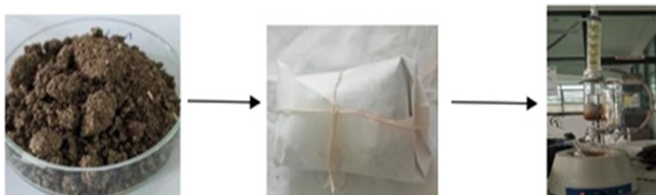
Figure 1. Sample preparation and maggot oil extraction process using the soxhlet method.
