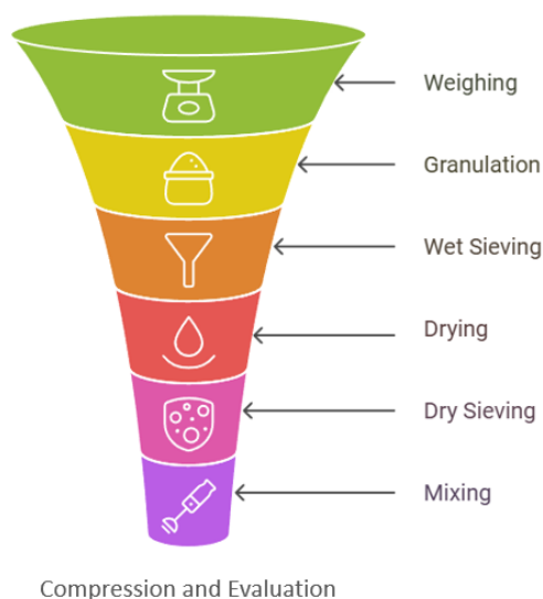
Figure 1. Flowchart of the preparation and testing of A. muricata leaf extract tablets
