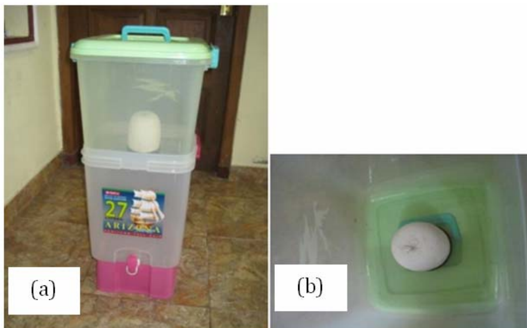
Figure 2 (a) Filtration test apparatus, (b) filter module.
