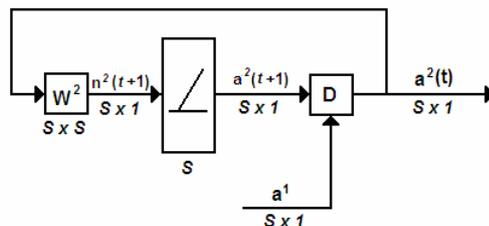
Figure 2. The Recurrent layer
