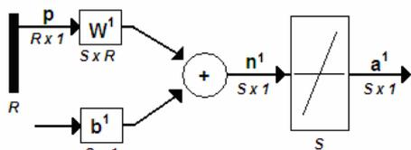
Figure 1. The Feedforward layer
