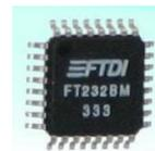
Gambar 8 *Chip Serial to USB*
