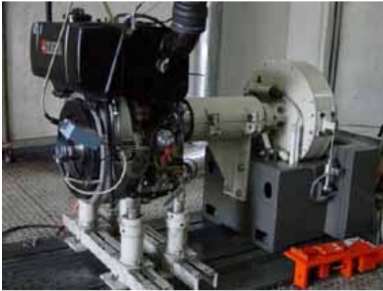
Gambar 3. Motor Bakar Research Diesel 1 silinder Hatz
