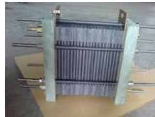
Gambar 4. Prototipe stack 20 cell.
