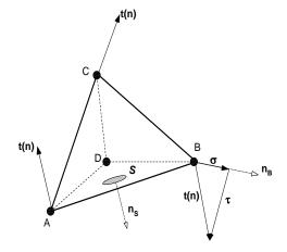
Figure 8. In VTK, a normal vector is defined directly at a surface e.g., n<sub>s</sub> at surface S, and tensor attributes is a property of point or grid, e.g., point or grid B
