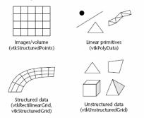
Figure 6. Type of data set supported by VTK (see VTK User's Guide)
