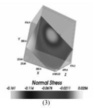
Figure 12. Different location of cutting plane inside a cube with a point load, i.e., positions (1), (2), and (3), shows the concentration of normal stress
