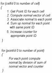
Figure 10. Procedure to obtain normal vector at a point (see VTK User's Guide book for explanation of the parameters).
