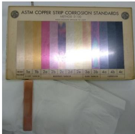
Gambar 4. Perbandingan ASTM Copper strip corrosion standard
