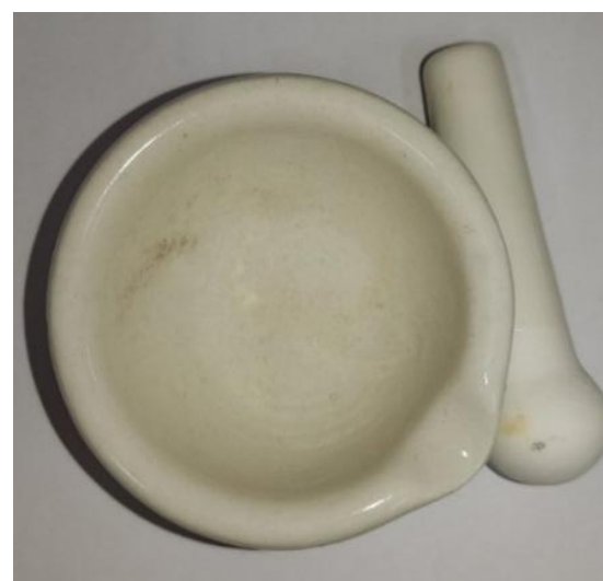
Figure 2. Previously used porcelain mortar exhibiting visible surface scratches
