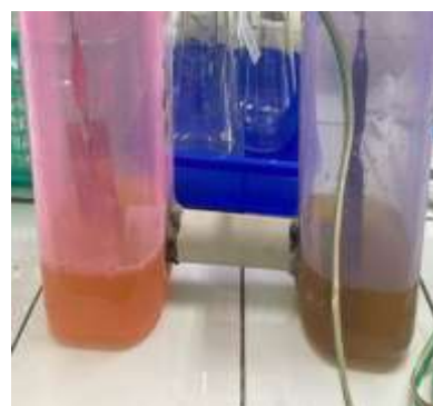
Figure 6. Schematic of the dual-chamber microbial fuel cell connected by an agar-salt bridge.
