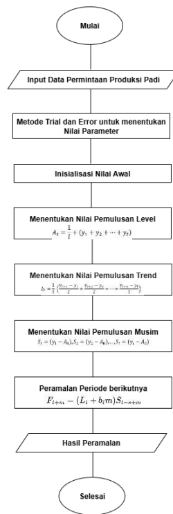
Gambar 1. Diagram Alir Metode Triple Exponential Smoothing
