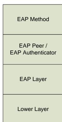
Figure 1. EAP layered-model
