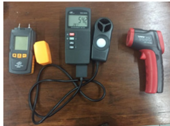
Figure 1. Infrared thermometer shafix WT380, Wood moisture tester GM605, dan Environment Meter EM-9000
