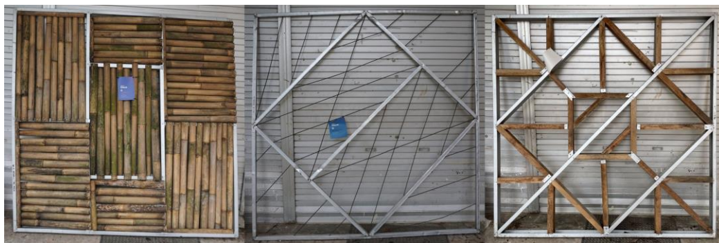
Figure 2. LGS Framed Wall Panels
