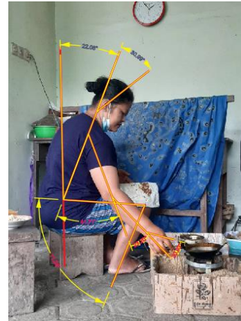
Figure 3. Withdrawal of the Working Posture of the Batik Maker When Filling the Canting Tool with the Wax
