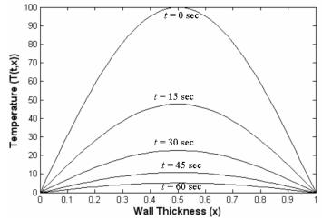
Figure 3. The temperature distribution obtained from Equation (8) along wall thickness during five time levels t = 0, 15, 30, 45, and 60 seconds
