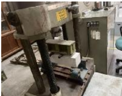
Figure 4. Flexural strength tests
