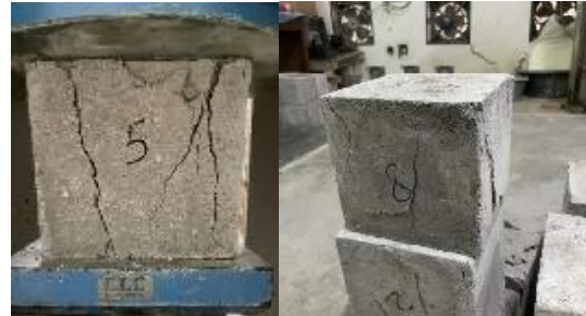
Figure 2. Samples compressive strength tests
